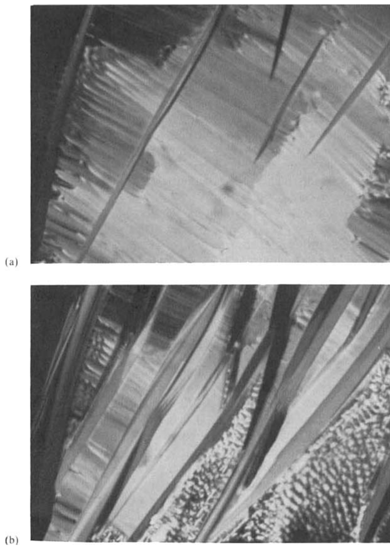
FIGURE 4 Growth of S_B spears in the S_A phase at 72.2^\circ (magnification = 10 \times 20 ) of
